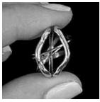
Bring band stamped "2" (other outside band) up against "1" band forming diamond shape. Note- these are the outside bands when the ring is assembled.
